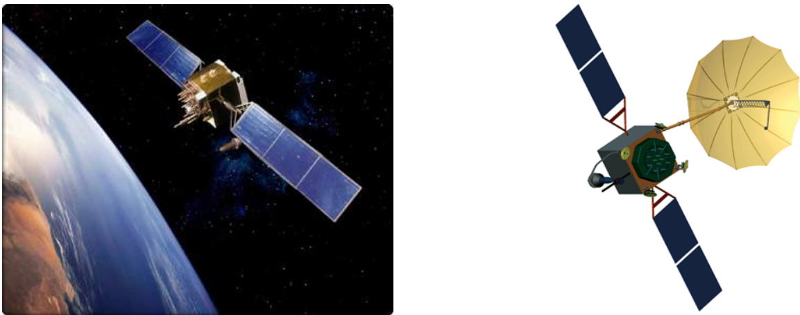
Figure 58: GPS IIF satellite (left) und GPS III satellite (right)
