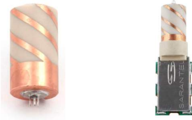
Figure 134: Passive (left) and active helix antenna
